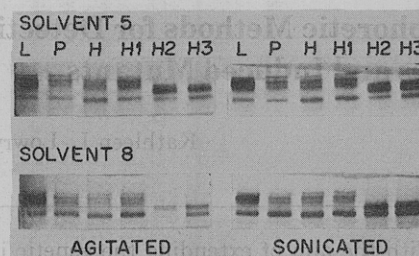
Figure 1. Electrophoretic patterns on gradient gels of soybean extracts in solvents 5 and 8 (Table I). Only the 6-9% portion of the gradient is shown. This portion contained the most intense bands and the only observable differences: L, Lee; P, Pickett; H, Harosoy; H1, H2, H3, mutants derived from Harosoy. The sample migrated from cathode to anode, or from the top to the bottom of the figure.
